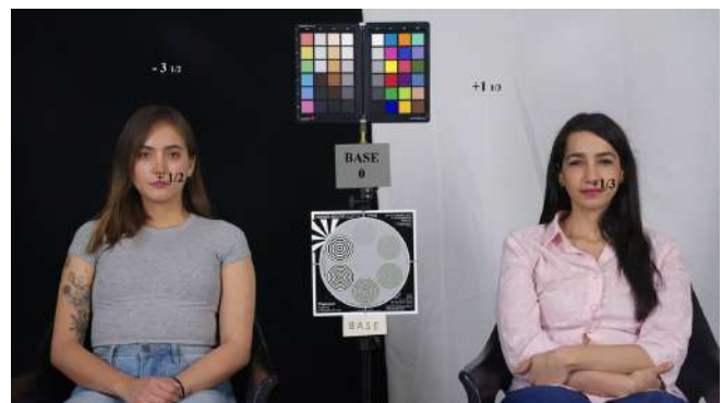
Comparison between the S-Cinetone and Slog3 curves at 4 stops overexposed and 4 stops underexposed.
