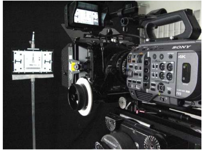
Resolution tests with ISO 12232 chart.
