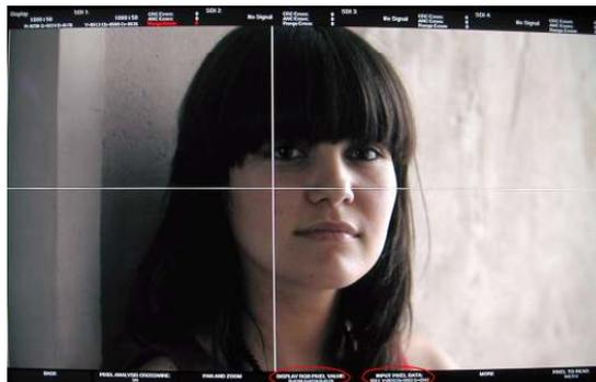
*Viewing the onscreen waveform monitor and vectorscope in different places. On the right, moveable cross hairs to measure pixel values that appear at the bottom of the screen.*
